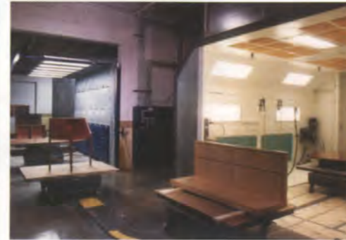
A variety of projects wend their way through Merritt's finishing room, which is equipped with a conveyorized cart system, three stages of ovens and a flash tunnel by Koch.
